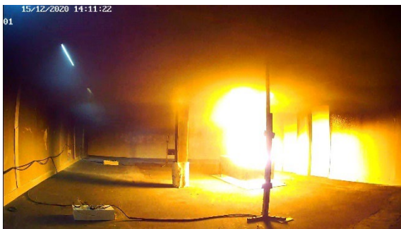
After 3'22" (activation 1 st sprinkler)
