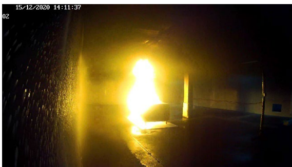
After 3'37" (activation 3 rd sprinkler)
