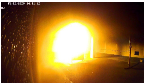
After 3'22" (activation 1 st sprinkler)
