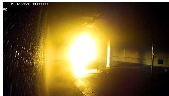
After 3'31" (activation 2 nd sprinkler)
