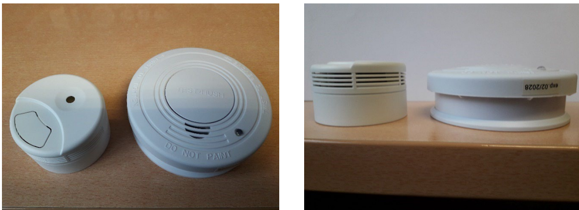
Figure 12: Optical smoke detectors of type FHB-150 Midi (left in each picture) and SA-19/1 (right in each picture)
