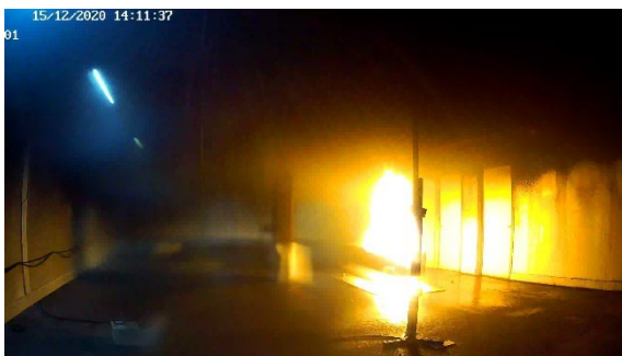
After 3'37" (activation 3 rd sprinkler)
